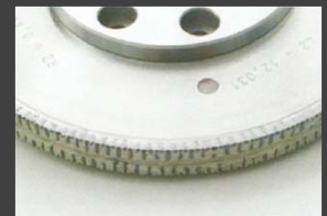
Diamond dressing roll in natural diamond for Gleason-Pfauter grinding machines. Diamond layer = elongated longs
