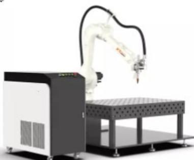
3D Fiber Laser Welding Robot
