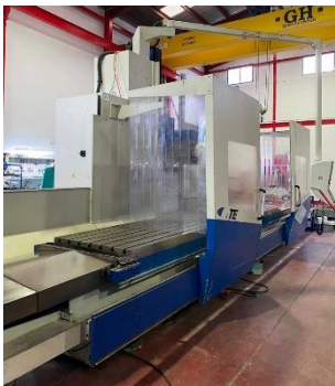
Fresadora MTE BF-4200. CNC HEIDENHAIN iTNC 530 Mesa: 4200x1000mm. Recorridos: 4000x1200x1500mm Cabezal automático. Cargador 20 htas y extractor. MTE BF-4200 milling machine. HEIDENHAIN iTNC 530 Table: 4200x1000mm. Travels: 4000x1200x1500mm Automatic head. Tool changer 20 units and conveyor
