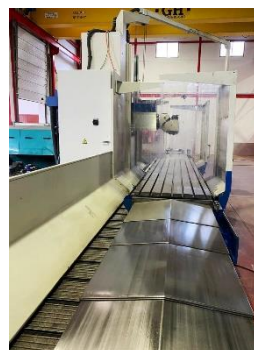
Fresadora MTE BF-4200. CNC HEIDENHAIN iTNC 530 Mesa: 4200x1000mm. Recorridos: 4000x1200x1500mm Cabezal automático. Cargador 20 htas y extractor. MTE BF-4200 milling machine. HEIDENHAIN iTNC 530 Table: 4200x1000mm. Travels: 4000x1200x1500mm Automatic head. Tool changer 20 units and conveyor
